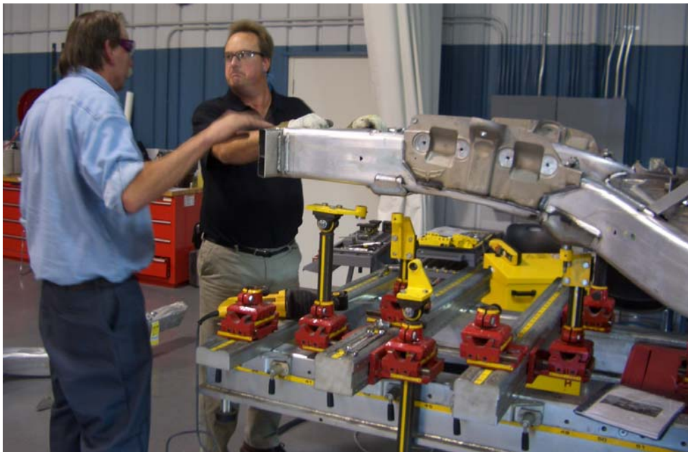
A Car Bench is used during the Z06/ZR1 Corvette class at the I-CAR Tech Center in Appleton, Wisconsin. At this point in the training, the universal jigs have been lowered in preparation for rail replacement.
